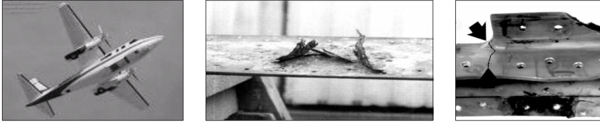
**Figure 4:** In the 1980s, division in CASA endangered Aero Commanders (left). The corrosion specialists let them fly for years with untreated exfoliation corrosion in their wing spars (centre). When the fatigue specialists found out, they stopped the practice, fearful that corrosion would worsen fatigue they were managing in the same spars (right – the arrows show a crack) [10]. We learned the lesson. One section now manages fatigue *and* corrosion.
